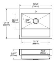
**Includes:** ELDSSF30279 sink, CTXBG2513R bottom grid, CTXDC0606 bottom grid drain cover, LKDD deep strainer drain
