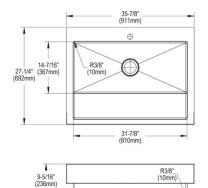
**Includes:** ELDSSF36279 sink, CTXBG3113R bottom grid, CTXDC0606 bottom grid drain cover, LKDD deep strainer drain
